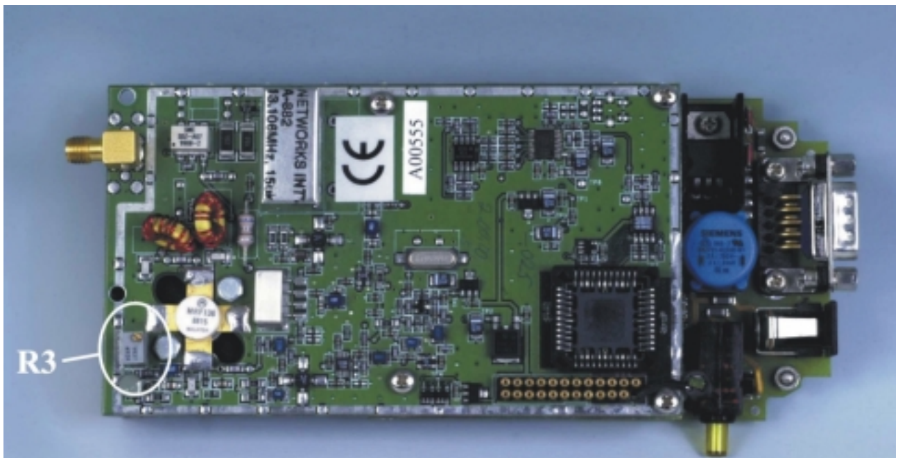
Figure 15: Location of Potentiometer R3 (RI-R00-321A)
